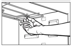
Unscrew the nut and lower the Browning / Broiling element. Use caution not to damage the Browning / Broiling element.
